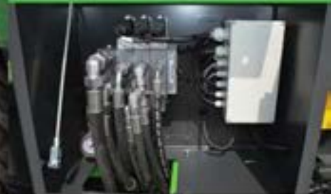
Hydraulic control block
