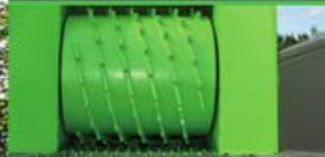
Top pressure roller Ø 520 mm
