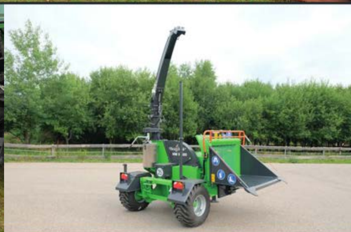
Discharge chute and flap electrical
