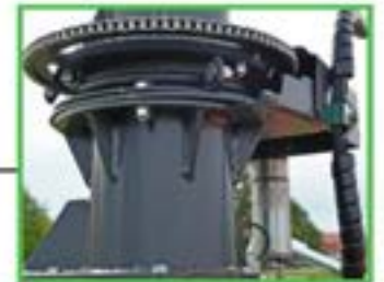
Discharge chute rotatable drive via electric motor
