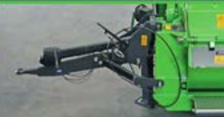
Hitch - height of towing port 500 mm
