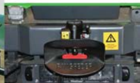
Automatic trailer coupling with compressed air connection
