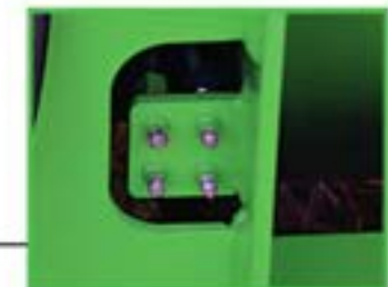
Central lubrication points easy and fast lubrication
