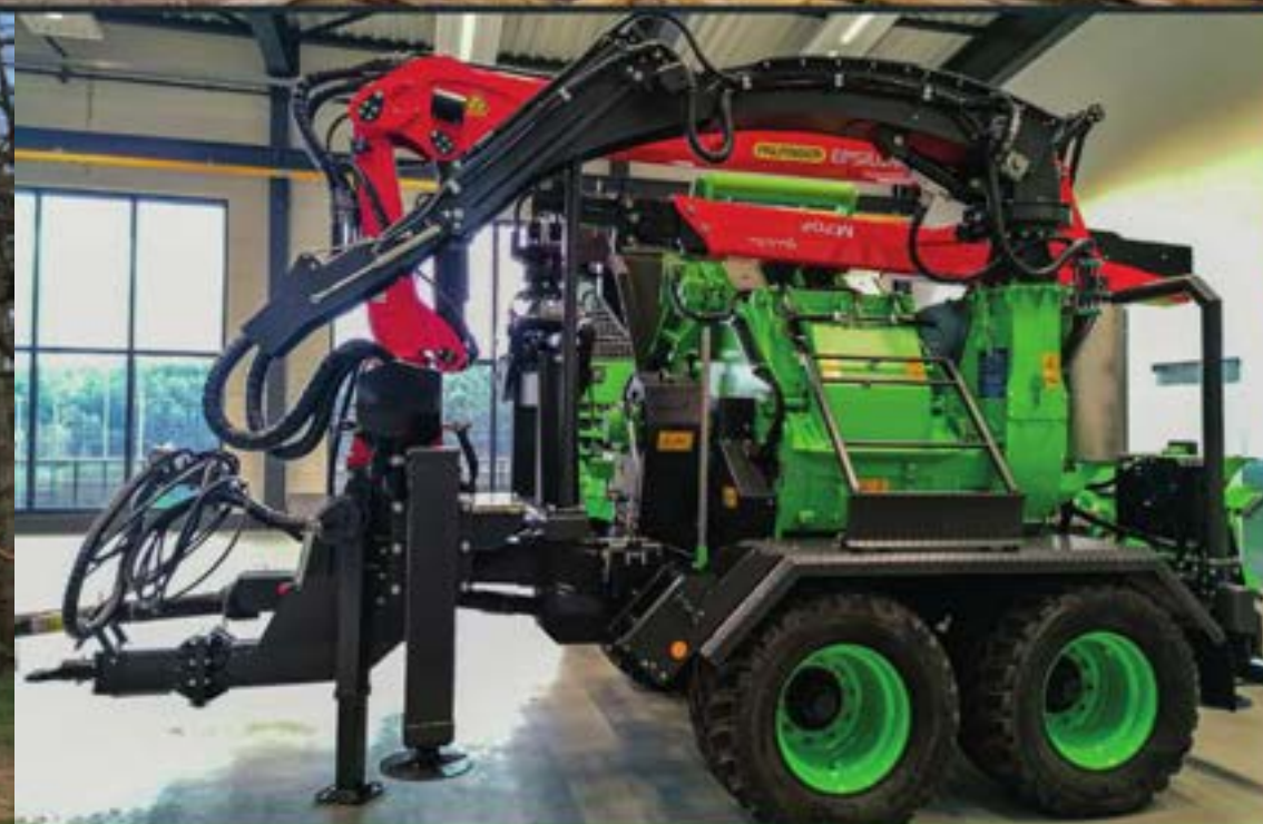
Automatic trailer coupling with compressed air connection
