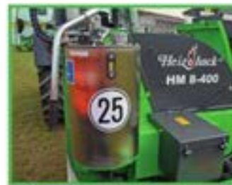
Height adjustable discharge chute with own oil supply hydraulically adjustable
